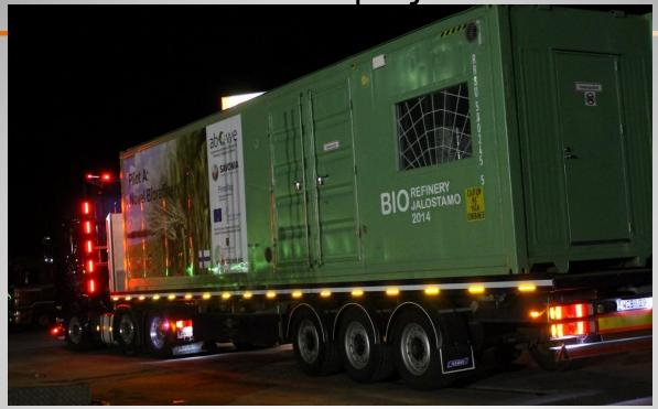
Movable ABOWE Pilot biorefinery unit for industry wastes, in Poland for potato industry and restaurant biowaste, and in Sweden for slaughterhouse wastes. The unit was constructed in Savonia University of Applied Sciences, Kuopio, Finland, under supervision of Adjunct Professor Elias Hakalehto. Photo: Mika Ruotsalainen.
